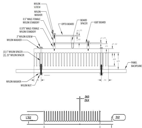
Figure 5: Heat Sink Drawing
