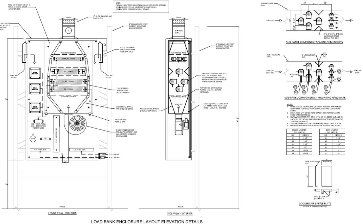
Figure 8: Load Bank Enclosure
